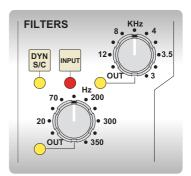
**DYN SC** – The Filters are switched into the sidechain of the Dynamics section. The Equaliser can be switched into the sidechain independently. Note that DYN SC overrides the INPUT function (see below).
